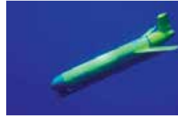
Teddy Webb's Slocum Thermal Glider deployed from the Virgin Islands and piloted by undergraduate summer interns.
